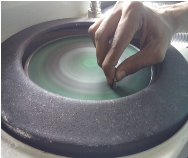
Fig 2.8 Fine polishing with Alumina Powder
